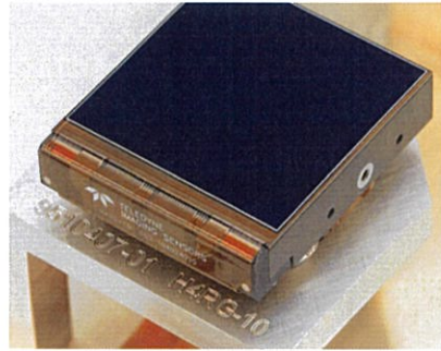
© Teledyne Imaging The 4096x4096 pixel HAWAII-4RG™
